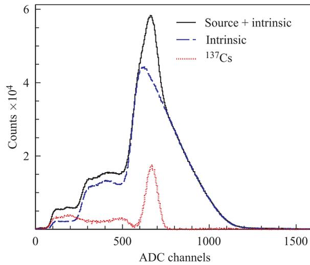
Fig. 6. The LYSO spectra due to intrinsic radioactivity and <sup>137</sup>Cs irradiation: total spectrum (solid line), spectrum due to intrinsic radioactivity (dashed line), and spectrum due to <sup>137</sup>Cs irradiation (dotted line)
