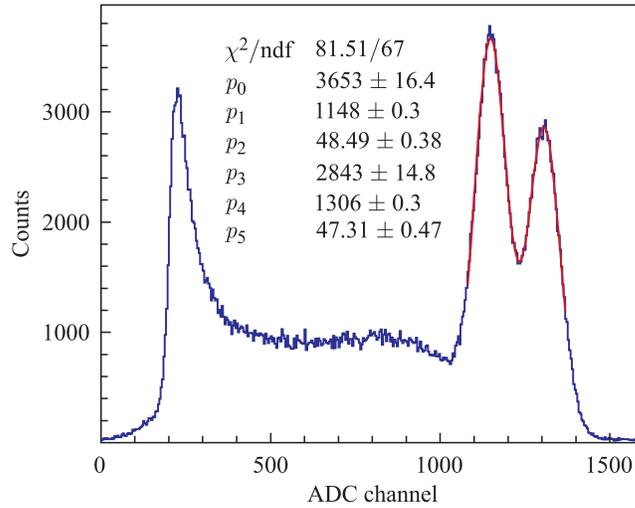
Fig. 7. The LYSO spectra due to  $^{60}\text{Co}$  irradiation. Two full absorption peaks corresponding to 1173 and 1333 keV are fitted with the sum of two Gaussians
