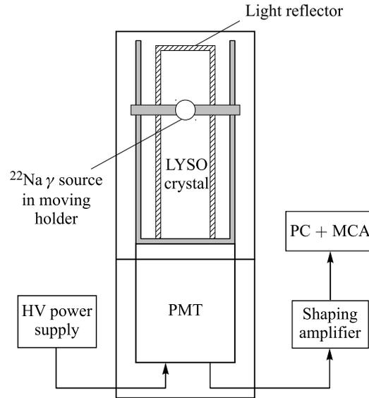
Fig. 2. The block diagram of the setup for measuring the  $30 \times 30 \times 130$  mm LYSO crystal light response uniformity
