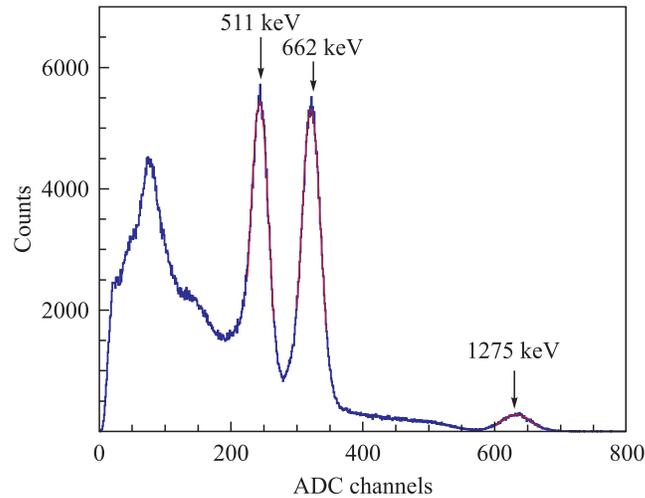
Fig. 13. The  $10 \times 10 \times 10$  mm LYSO crystal spectrum due to intrinsic radioactivity and  $^{22}\text{Na}$  and  $^{137}\text{Cs}$  irradiation. Three full absorption peaks are fitted with Gaussians
