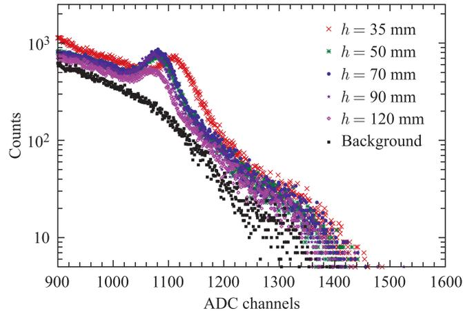
Fig. 10. Pulse height spectra of the  $30 \times 30 \times 130$  mm LYSO crystal irradiated by the  $^{22}\text{Na}$   $\gamma$  source placed at distances of 35, 50, 70, 90 and 120 mm from the PMT cathode (1786 keV peaks are around channel 1100)
