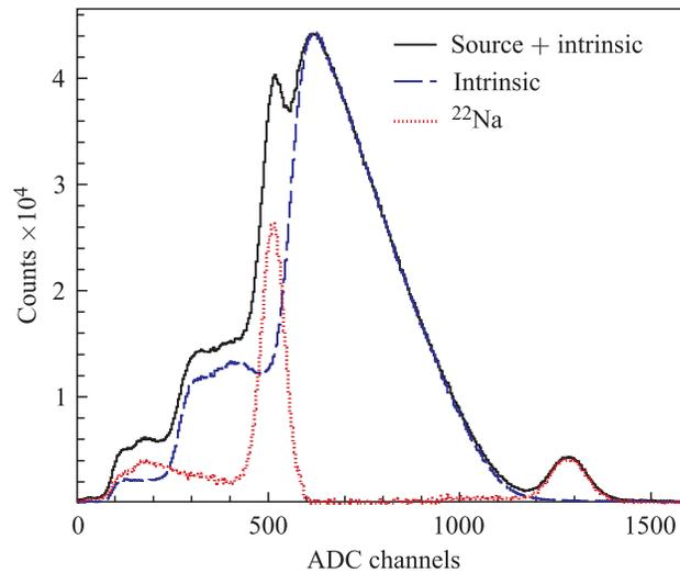
Fig. 5. The LYSO spectra due to intrinsic radioactivity and  $^{22}\text{Na}$  irradiation: total spectrum (solid line), spectrum due to intrinsic radioactivity (dashed line), and spectrum due to  $^{22}\text{Na}$  irradiation (dotted line)
