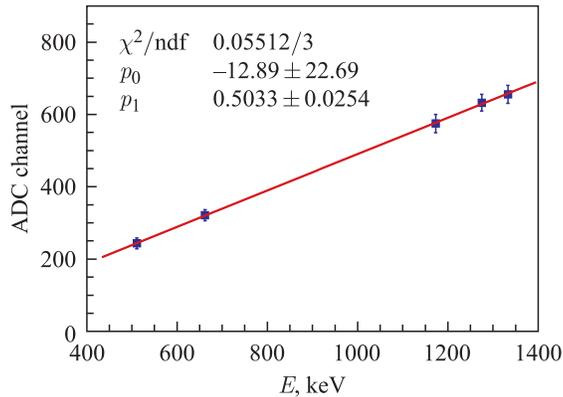
Fig. 15. The  $10 \times 10 \times 10$  mm LYSO crystal energy response linearity in the 511–1333 keV range measured by the S8664-1010 Hamamatsu APD
