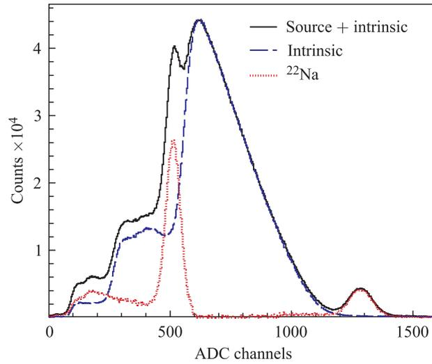
Fig. 5. The LYSO spectra due to intrinsic radioactivity and <sup>22</sup>Na irradiation: total spectrum (solid line), spectrum due to intrinsic radioactivity (dashed line), and spectrum due to <sup>22</sup>Na irradiation (dotted line)
