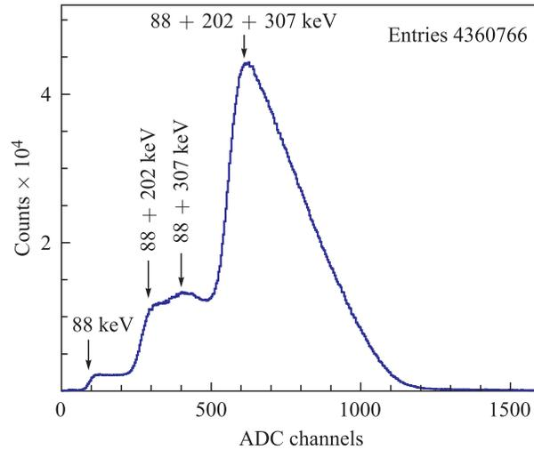
Fig. 4. The  $30 \times 30 \times 130$  mm LYSO crystal spectrum due to intrinsic radioactivity. Four sets of detected gammas are shown in the spectrum by arrows
