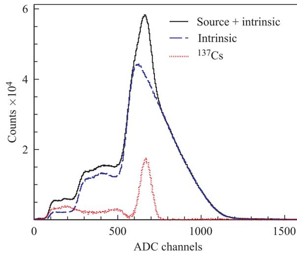
Fig. 6. The LYSO spectra due to intrinsic radioactivity and  $^{137}\text{Cs}$  irradiation: total spectrum (solid line), spectrum due to intrinsic radioactivity (dashed line), and spectrum due to  $^{137}\text{Cs}$  irradiation (dotted line)
