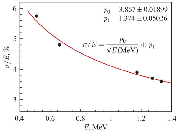
Fig. 8. The  $30 \times 30 \times 130$  mm LYSO crystal energy resolution measured with the EMI 9813B PMT as a function of photon energy
