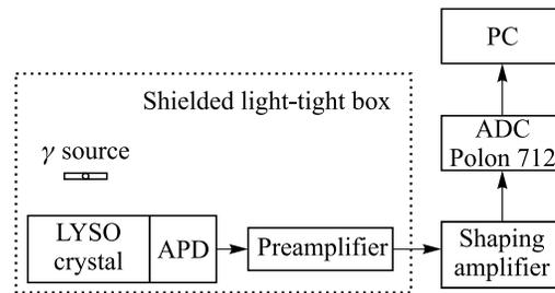
Fig. 3. The block diagram of the setup for measuring the  $10 \times 10 \times 10$  mm LYSO crystal energy resolution
