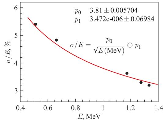
Fig. 14. The  $10 \times 10 \times 10$  mm LYSO crystal energy resolution measured by the S8664-1010 Hamamatsu APD as a function of the photon energy
