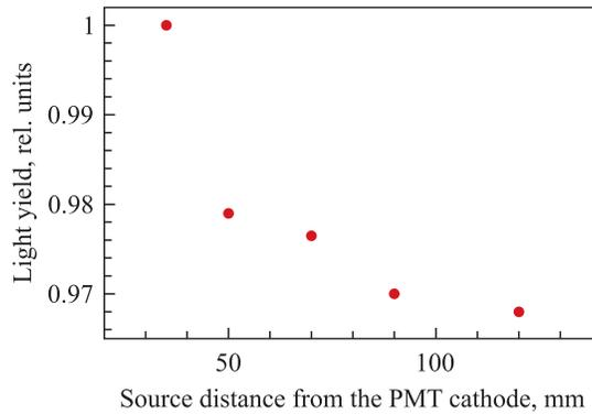
Fig. 11. Longitudinal light response uniformity of the  $30 \times 30 \times 130$  mm LYSO crystal. Nonuniformity does not exceed 3.2% for the  $\gamma$ -source position ranging between 35 and 120 mm on the crystal axis
