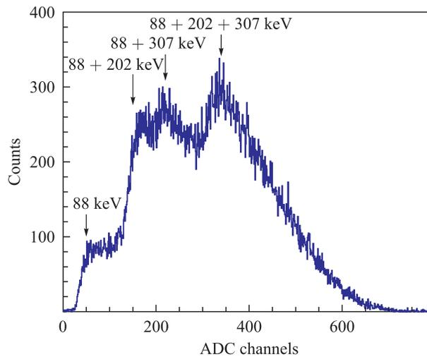
Fig. 12. The  $10 \times 10 \times 10$  mm LYSO crystal spectrum due to intrinsic radioactivity measured with the S8664-1010 Hamamatsu APD. Four sets of detected gammas are shown in the spectrum by arrows
