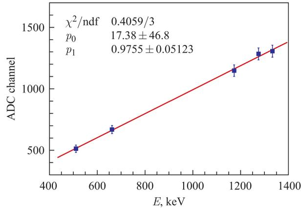
Fig. 9. The  $30 \times 30 \times 130$  mm LYSO crystal energy response linearity in the 511–1333 keV range
