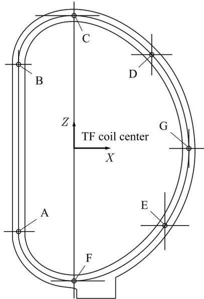
Fig. 2. Locations of the reference points A–G on the TF coil centreline
