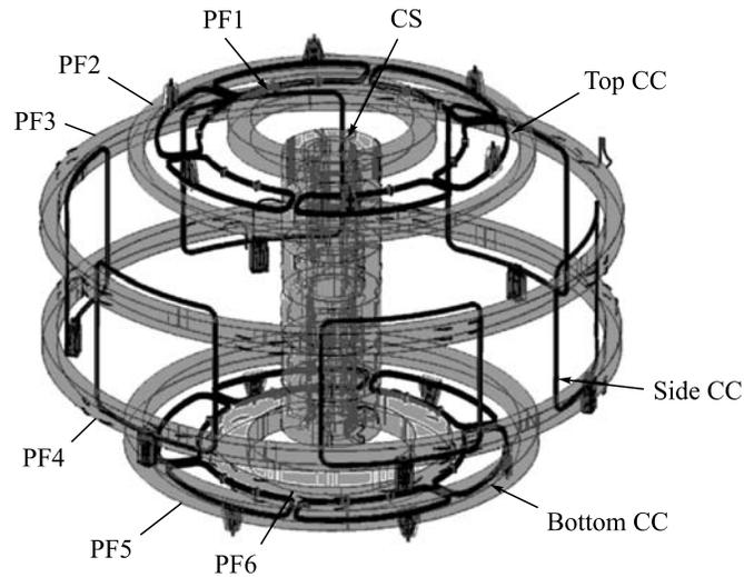
Fig. 1. Layout of correction coils, PF and CS coils
