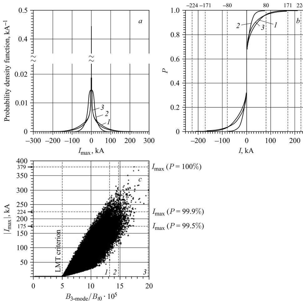
Fig. 3. Probability distributions of the CC currents (*a*), integrated probability of required currents (*b*), and required currents in the Bottom CC (*c*). 1 — Top CC; 2 — Side CC; 3 — Bottom CC. SOF conditions, 670 DOF, *increased tolerances*, 1,000,000 statistical events. Root-mean-square norm (2)
