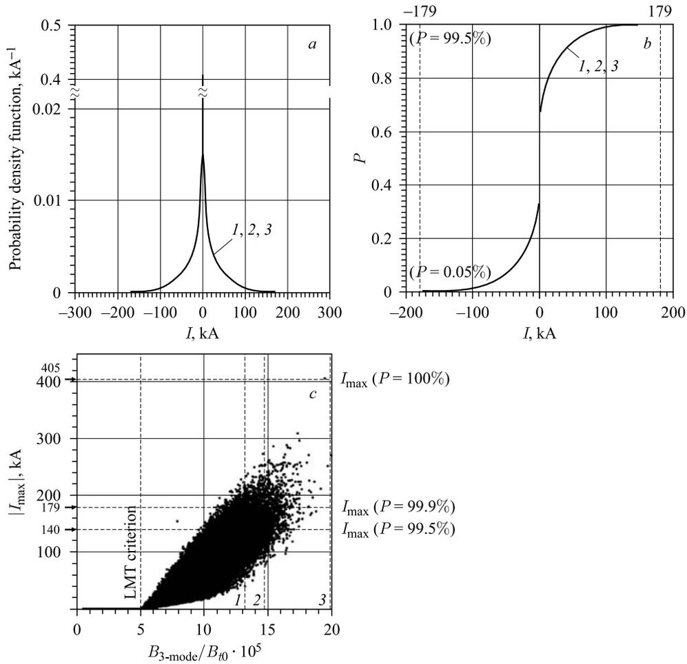
Fig. 4. Probability distributions of the CC currents (a), integrated probability of required currents (b), and required currents in the Bottom CC (c). 1 — Top CC; 2 — Side CC; 3 — Bottom CC. SOF conditions, 670 DOF, increased tolerances, 1,000,000 statistical events. Norm of the lowest of a set of maximum currents (3)
