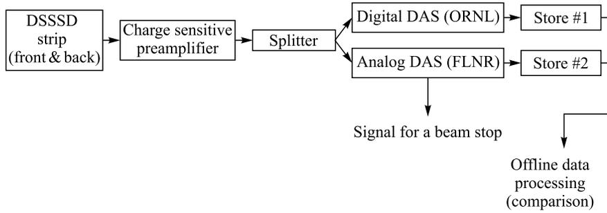
Fig. 2. Block diagram of the spectrometer of the DGFRS
