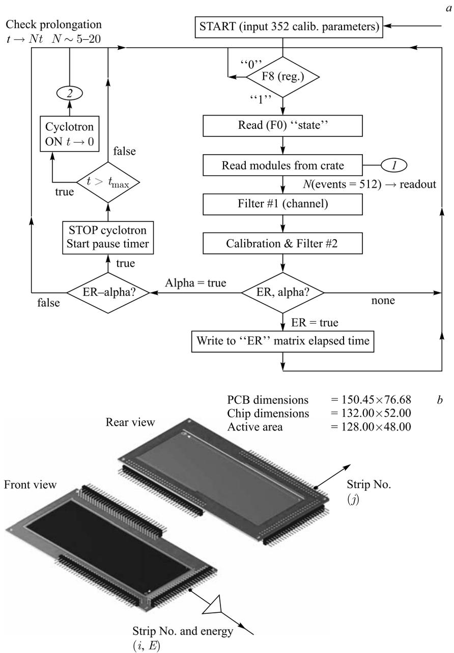
Fig. 6. *a*) The flowchart of the data taking process and ER-alpha searching (*1* — check beam off pause prolongation; *2* — file writing). *b*) Schematic of ER matrix element (ER elapsed time  $t_{i,j;ER=true}$ ) formation. View (front and rear) of DSSSD detector of the DGFRS
