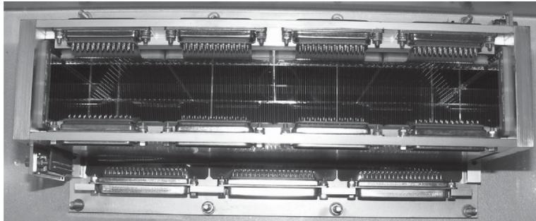
Fig. 1. Si strip detector of the well type
