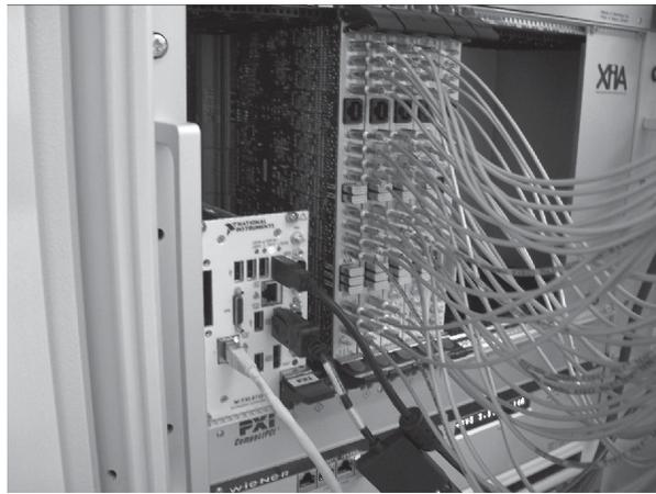
Fig. 3. PXI chassis with XIA digitizers and a NI controller
