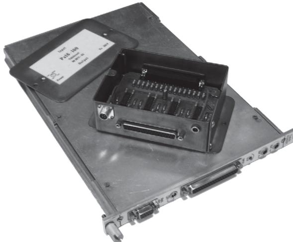
Fig. 2. Multichannel preamplifier and multiplexer-amplifier
