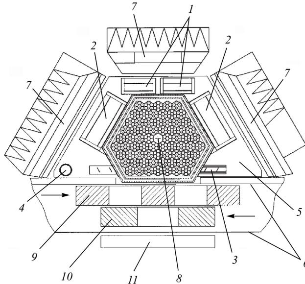
Fig. 1. Cross-sectional view of the IBR-2M core: 1 — emergency protection blocks; 2 — compensation block; 3 — intermediate control block; 4 — automatic regulator; 5 — stationary reflector; 6 — moving reflector jacket; 7 — grooved water moderators; 8 — external neutron source; 9 — MMR; 10 — AMR; 11 — flat water moderator
