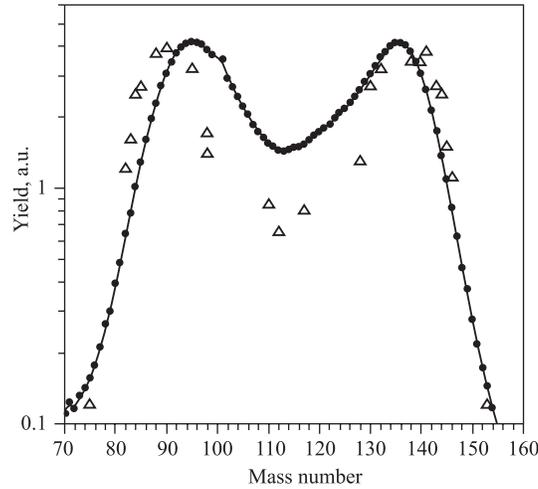
Fig. 2. Comparison of  $M_{te}$  spectra obtained in this work (circles) and  $M_{te}$  spectra from the reaction  $^{232}\text{Th} + d$  (11.5 MeV) [6] (triangles). The latter were obtained by radio-chemical method
