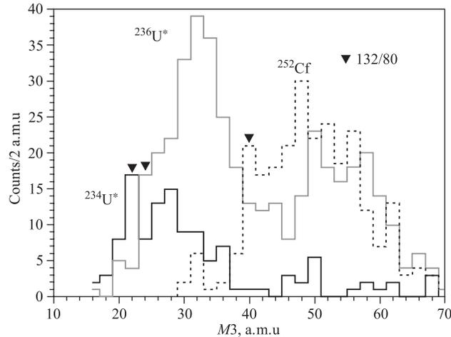
Fig. 6. Mass spectra of the lightest fragment in ternary fission of three different fissioning systems [10]. Triangles mark the partitions corresponding to the fixed difference  $M_c - M_3 = 212$  a.m.u. presumably linked with total mass of magic clusters of  $^{132}\text{Sn}$  and  $^{80}\text{Ge}$
