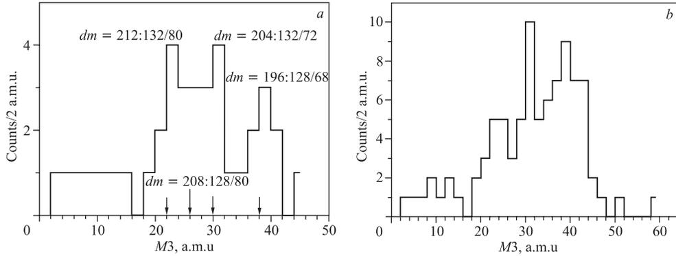
Fig. 5. *a*) Mass spectrum of the lightest fragments in each detected triplet of fragments under condition  $M_s < 242$  a.m.u. (see Fig. 4, *b*). *b*) Similar spectrum for all ternary events detected. The arrows in the figure mark the partitions based on pairs of known magic nuclei of Ni, Ge, Sn
