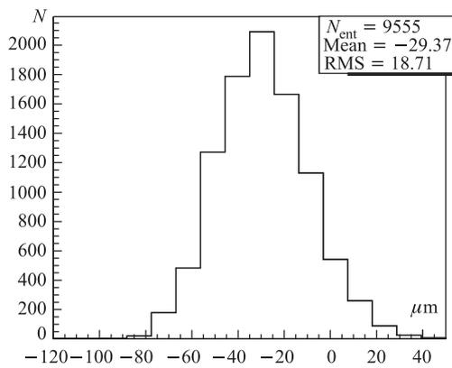
Fig. 4. Panels thickness deviation
