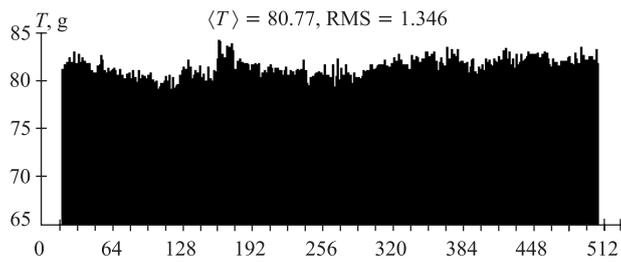
Fig. 3. Typical wires tension for one layer
