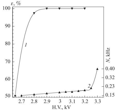
Fig. 8. Layer track registration efficiency  $\varepsilon$  (1) and noise  $N$  (2) vs. high voltage
