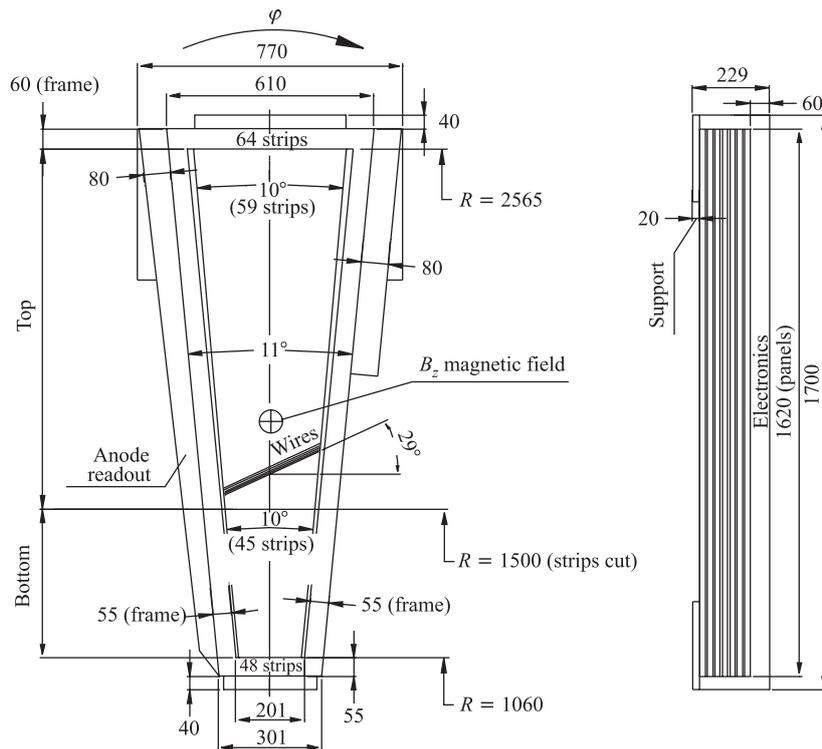
Fig. 2. Overall dimensions of ME1/1 CSC (in millimeters)
