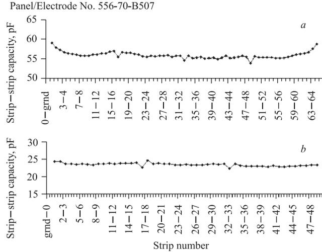
Fig. 5. Typical strip–strip capacity for one layer: a) top; b) bottom
