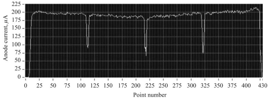
Fig. 7. Example of the current scan along tested TRD chamber with the X-ray source
