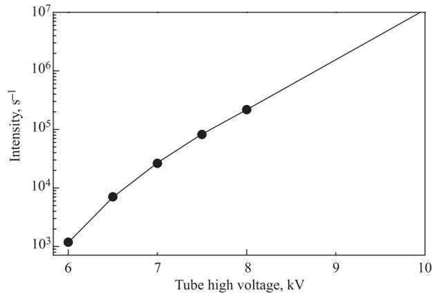
Fig. 6. The intensity of X-ray photons behind the radiator as a function of the tube high voltage, the tube current — 100  $\mu$ A
