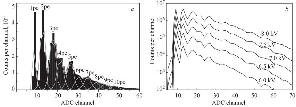
Fig. 5. Pulse height distributions measured with the scintillation detector. *a*) The tube HV = -8 kV, the curves — the Gaussian multiple-peak fit. *b*) The amplitude spectra obtained with different magnitudes of the tube high voltage
