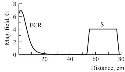
Fig. 2. Longitudinal magnetic field in the beam line
