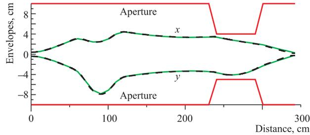
Fig. 22. Horizontal ( $x$ ) and vertical ( $y$ )  $^{40}\text{Ar}^{7+}$  beam envelopes. Dashed line — moments method; solid line — macro particles
