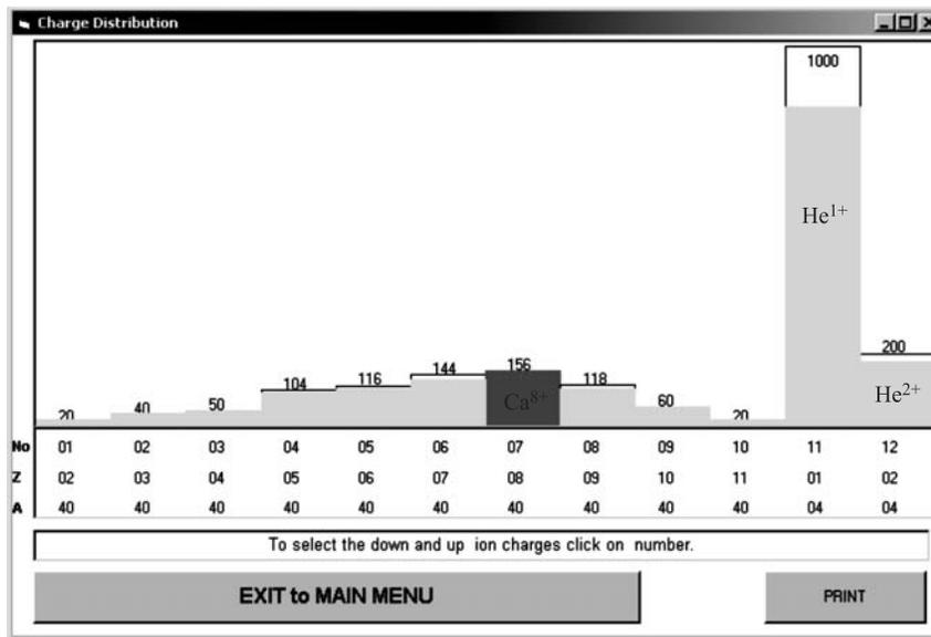
Fig. 14. The spectrum of the  $^{40}\text{Ca}$  and helium ions beam. The designations are the same as in Fig. 3
