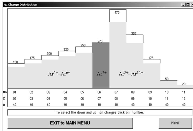
Fig. 3. Argon beam spectrum. Total beam current — 2.31 mA. No — ordinal number of the ion species; Z, A — charge and mass of the ion. Upper numbers are the currents of the different charge states of the beam in  $\mu A$
