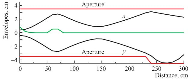
Fig. 16. Horizontal ( $x$ ) and vertical ( $y$ ) envelopes of the  $^{40}\text{Ca}^{8+}$  ion beam
