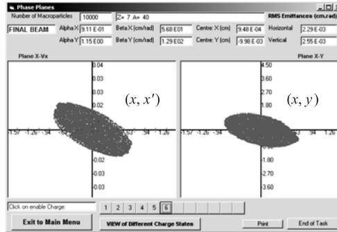
Fig. 9. The  $^{40}\text{Ar}^{7+}$  ions distributions just after the analyzing magnet
