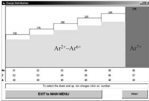
Fig. 8. Argon beam spectrum with lower charge states. The designations are the same as in Fig.3
