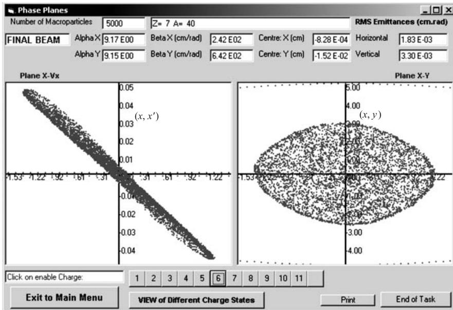
Fig. 24. The  $^{40}\text{Ar}^{7+}$  ions distributions just after the analyzing magnet. Electrostatic triplet focusing
