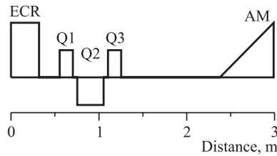
Fig. 20. Scheme of the triplet focusing. Q1–3 — electrostatic lenses
