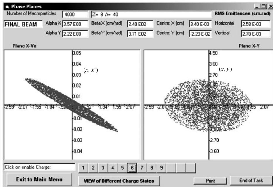
Fig. 19. The  $^{40}\text{Ca}^{8+}$  ions distributions just after the analyzing magnet. Calcium beam transportation without helium beam
