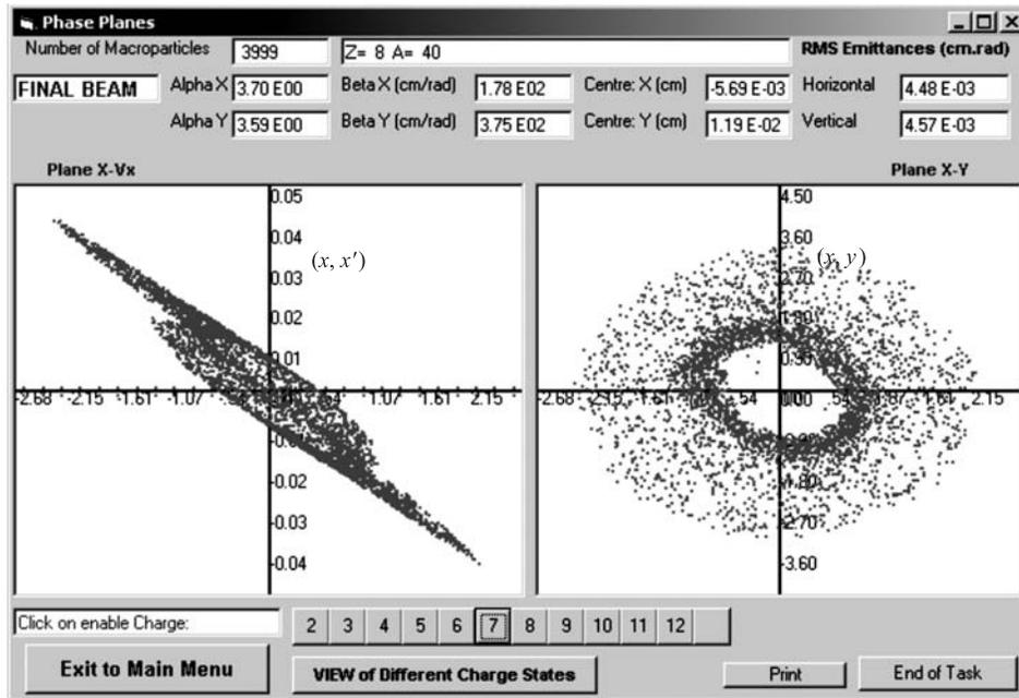
Fig. 18. The  $^{40}\text{Ca}^{8+}$  ions distributions just after the analyzing magnet. Calcium beam transportation with helium beam
