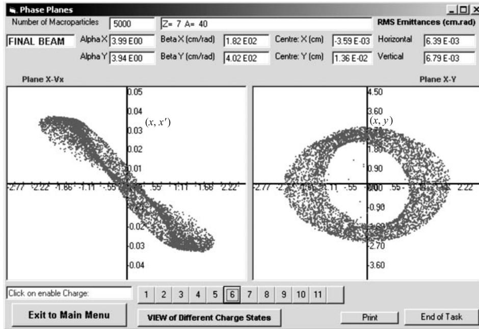
Fig. 7. The  $^{40}\text{Ar}^{7+}$  ions distributions just after the analyzing magnet
