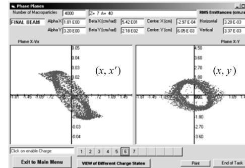
Fig. 13. The  $^{40}\text{Ar}^{7+}$  ions distributions just after the analyzing magnet
