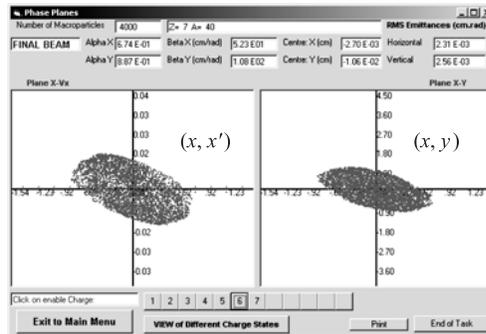
Fig. 11. The  $^{40}\text{Ar}^{7+}$  ions distributions just after the analyzing magnet
