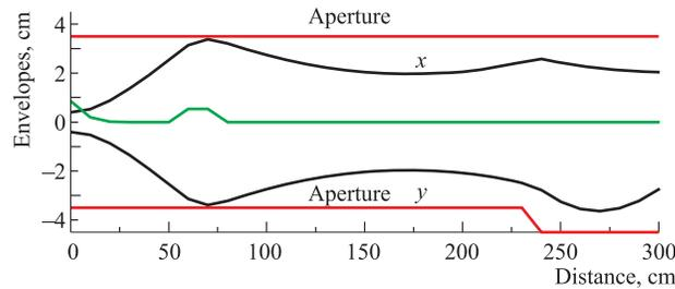
Fig. 5. Horizontal ( $x$ ) and vertical ( $y$ ) envelopes of the  $^{40}\text{Ar}^{7+}$  ion beam
