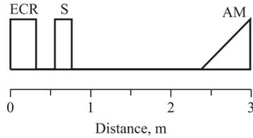
Fig. 1. Scheme of the beam line: ECR — longitudinal magnetic field of the ECR-ion source; S — focusing solenoid; AM — 90° analyzing magnet
