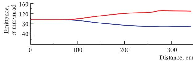
Fig. 23. Horizontal ( $x$ ) and vertical ( $y$ ) emittances of the  $^{40}\text{Ar}^{7+}$  beam
