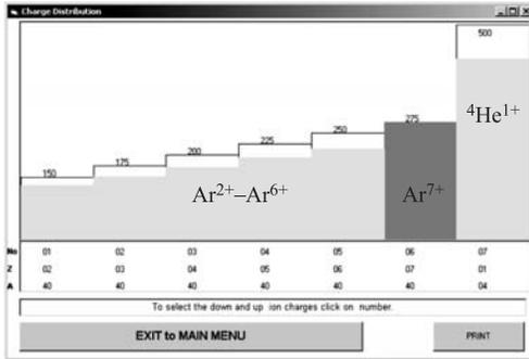
Fig. 12. Argon and  $^4\text{He}^{1+}$  beam spectrum. The designations are the same as in Fig.3
