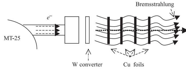
Fig. 1. The experimental setup for bremsstrahlung photon flux determination
