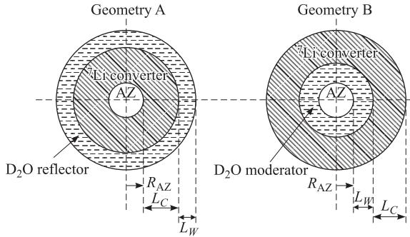
Fig. 2. Geometry of the multilayer converter
