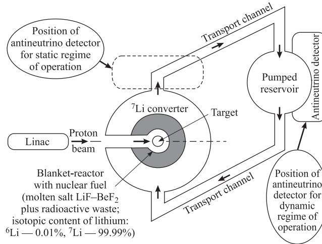
Fig. 3. Scheme of the lithium antineutrino source on the basis of the booster-type neutron source. Variants for the static and dynamic regimes of operation
