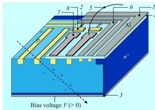
Fig. 2. The CMS silicon strip sensor [4]: 1 — guard ring (ground); 2 — bias resistor (poly); 3 — Al backplane; 4 —  $\text{SiO}_2$  layer; 5 — bond wire; 6 — bias ring; 7 — AC pad; 8 — DC pad
