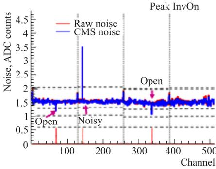
Fig. 5. Bad channels identified by LT test in the noise analysis
