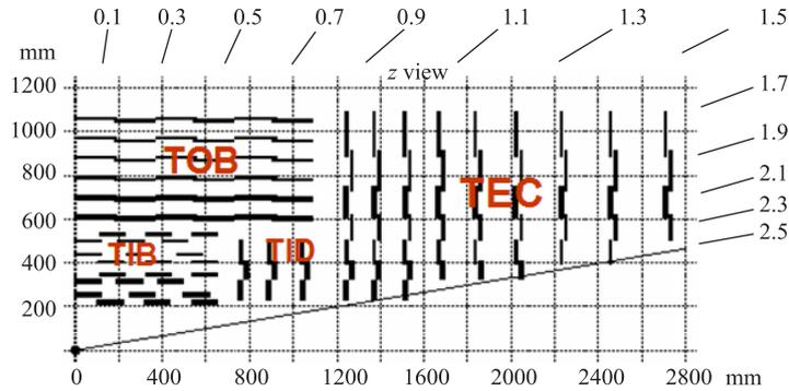
Fig. 1. A quarter view of CMS SMT. Locations of the subtrackers and number of layers are seen from the figure. Thin and thick lines represent the single- and double-sided modules, respectively. Top axis belongs to pseudorapidity
