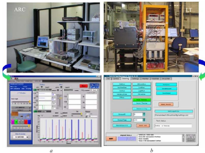
Fig. 4. ARC (a) and LT (b) systems for module testing
