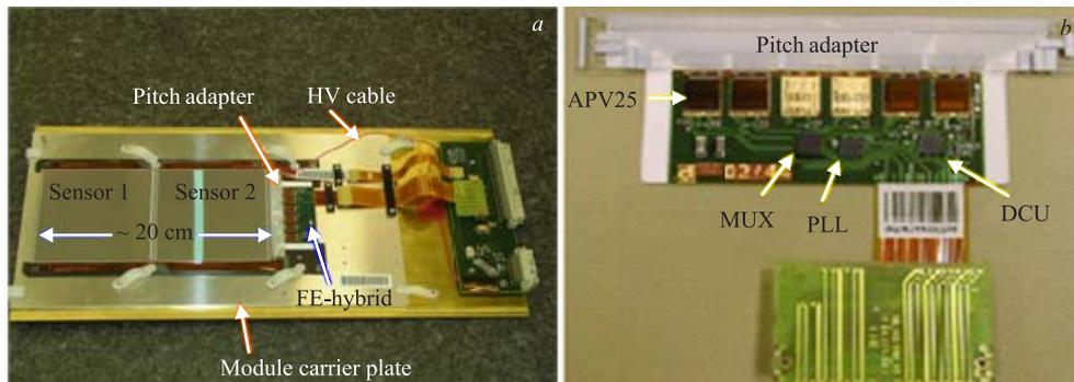
Fig. 3. CMS TOB silicon detector module (a) and close view of the front-end hybrid (b)
