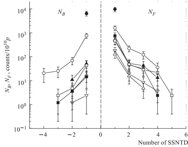
Fig. 2. The registered numbers of counts in front and back hemispheres for 1-GeV protons and the assembly with sections P-10D-T-10D-P. On the horizontal axis the zero corresponds to a position of the target, and numbers specify a number of SSNTD counted from the target. The symbols denote experimental data:  $\nabla$  — Al;  $\Delta$  — PVC;  $\blacktriangle$  — Ti;  $\blacksquare$  — Cu;  $\square$  — Cd;  $\circ$  — Ta;  $\bullet$  — Pb; the curves — result of fitting
