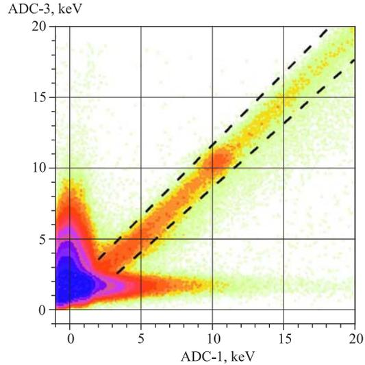
Fig. 2. Example of the primitive Fourier analysis done with two different shaping times: ADC-1 operates with  $2 \mu\text{s}$  pulses, and ADC-3 operates with  $12 \mu\text{s}$  pulses. (Color intensity scale is logarithmic)
