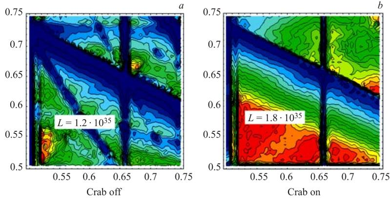
Fig. 4. A luminosity scan by LIFETRACK. Axes are the betatron tunes. The red color corresponds to the highest luminosity while the blue is the lowest one
