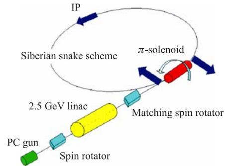
Fig. 7. TCF spin manipulation schematically
