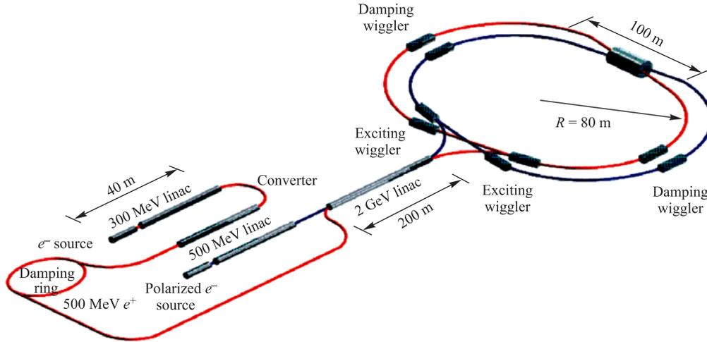
Fig. 3. Schematic view of the Novosibirsk TCF
