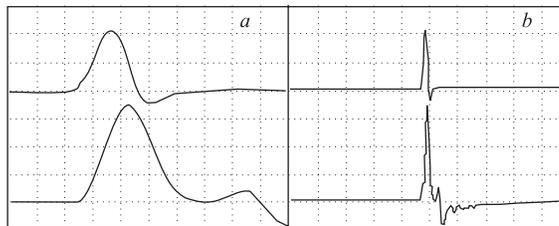
Fig. 5. Input current (upper trace) and output pulse (lower trace). *a*) 2.5 ns/div; *b*) 25 ns/div
