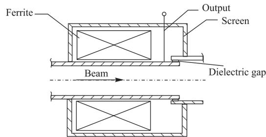
Fig. 1. Conceptual design of the monitor
