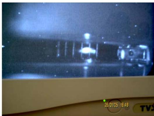
Fig. 6. Photo of the extracted beam of  $^{86}\text{Kr}^{15+}$  after magnetic channel. The distance between wires is 5 mm
