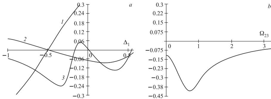
Fig. 2. a) Phase shift via detuning  $\Delta_1$ : 1 — for  $|100\rangle$ -state; 2 — for  $|110\rangle$ -state; 3 — for  $|111\rangle$ -state. b) Phase shift for  $|111\rangle$ -state via Rabi frequency  $\Omega_{23}$
