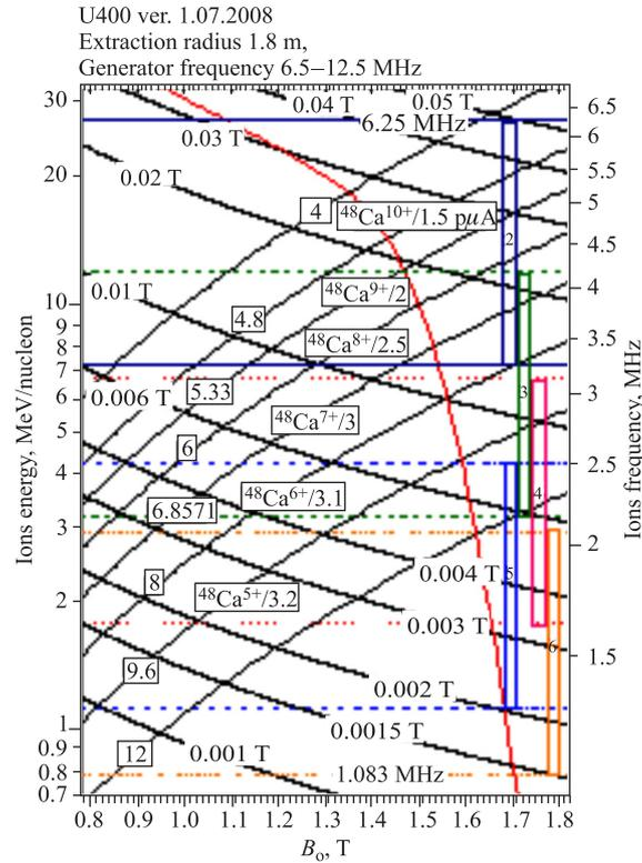
Fig. 3. Operating chart of the U400R cyclotron
