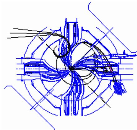
Fig. 5. Scheme of beam extraction from U400M
