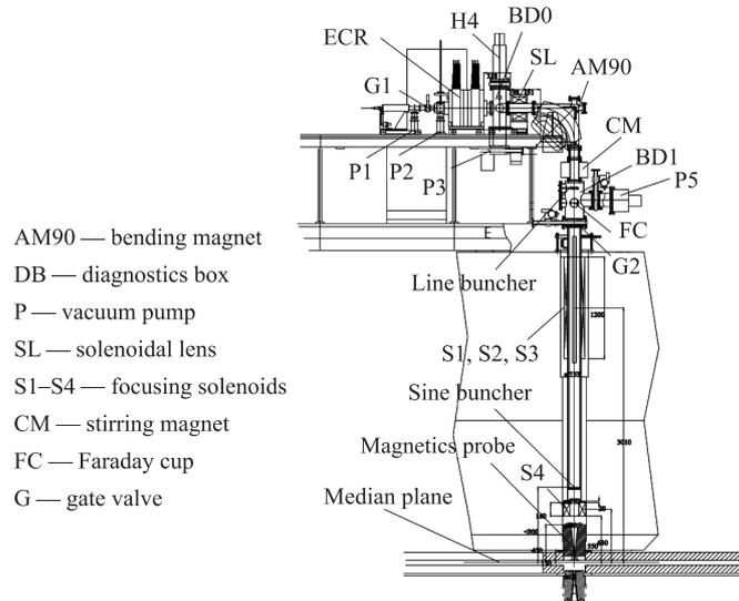
Fig. 7. U400R axial injection system
