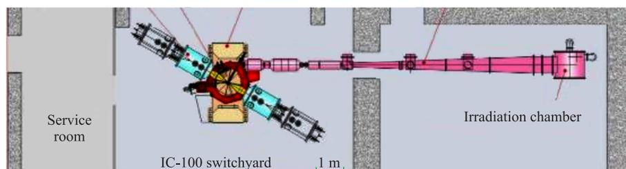
Fig. 6. Plan of a specialized complex for applied research based on the IC-100 cyclic implanter
