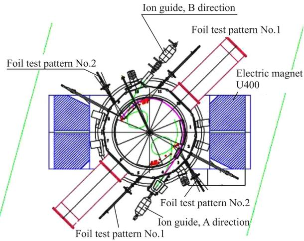
Fig. 4. Scheme of the beam extraction from U400R in two directions
