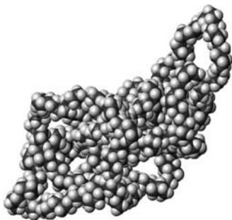
Fig. 1. Initial configuration of a flexible polyethylene chain
