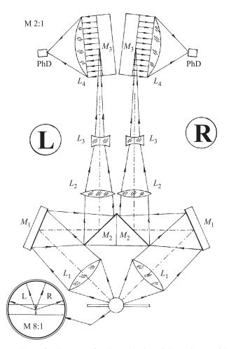
Fig. 4. Stereoscopic confocal scanner for the vertical particle tracks, provided with two confocal scanners on both sides of view (L and R):  $L_1$  — two main imaging lenses,  $L_2$  and  $L_3$  — two pair of Newton monocular lenses,  $L_4$  — two collecting lenses,  $M_1$  — two first-plane mirrors,  $M_2$  — two second-plane mirrors,  $M_3$  — two orthogonalization mirrors, PhD — two point-like photodiodes
