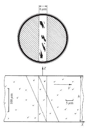
Fig. 1. The results of the experimental testing of the dark-field confocal scanning microscope for selective observation of the vertical particle tracks. Top: signals of four particle tracks inside the illuminating zone of  $6\,\mu\text{m}$  width. Bottom: the cross section of the same region
