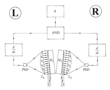
Fig. 5. Coincidence electronic circuit for two output signals from the stereoscopic confocal scanner for vertical particle tracks:  $M_3$  — two orthogonalization mirrors, PhD — two point-like photodiodes, d/dt — time differentiation circuit, AND — coincidence electronic circuit, S — storage block
