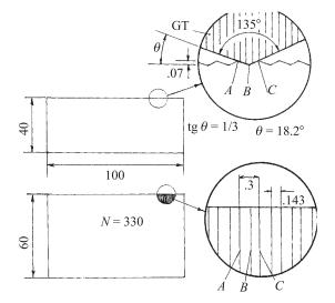
Fig. 3. Image orthogonalization system: GT — grooving tool; A, B and C are three points of the lamelar region, BC is the working part of the lamelar mirror. All dimensions — in mm
