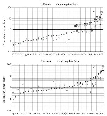
Fig. 2. Enrichment factors (EF) of elements in moss, sampled at Zemun and Kalemegdan Park, calculated to: *a*)  $\text{EF} = [\text{E/Al}]_{\text{moss}} / [\text{E/Al}]_{\text{Crust}}$ , the crustal element composition given by Mason (1966) [30]; *b*)  $\text{EF} = [\text{E/Al}]_{\text{moss}} / [\text{E/Al}]_{\text{topsoil}}$ , the concentration of elements in local topsoil determined in this study
