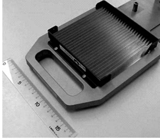
Fig. 3. A bar ridge filter for the therapeutic proton beam
