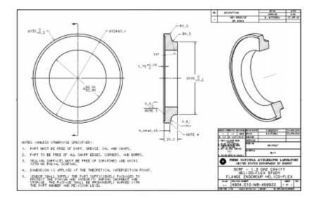
Fig. 1. Endgroup flange made of Nb-Ti
