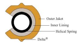
Fig. 12. Garlock Helicoflex Delta seal
