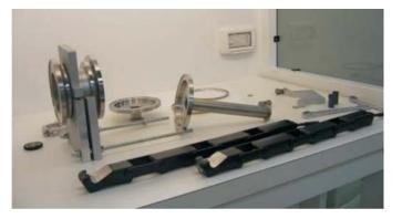
Fig. 13. Set-up for the contamination measurements of sample N1 in the Pisa clean room
