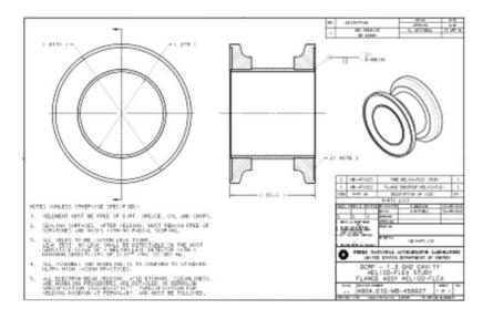
Fig. 3. Endgroup structure assembly
