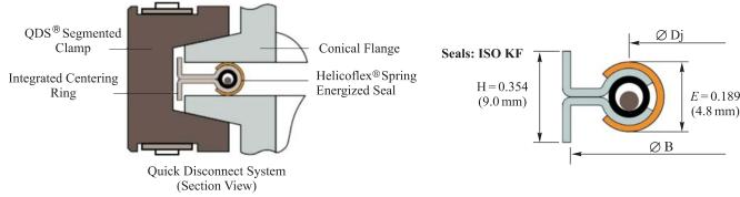
Fig. 10. Detail of the Garlock QDS + Helicoflex
