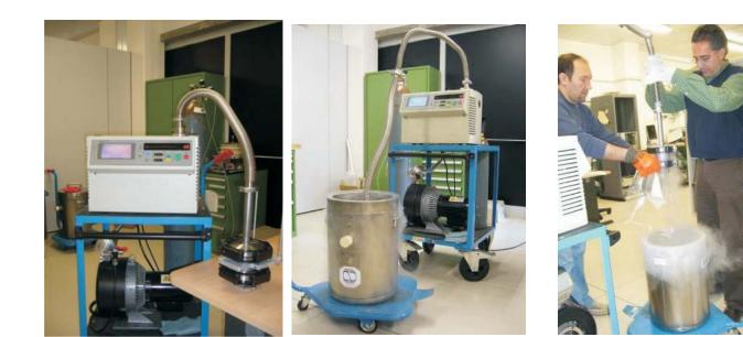
Fig. 18. The sample N1 He-leak test at room temperature
