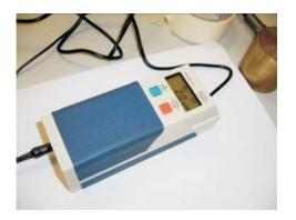
Fig. 6. Mitutoyo surface roughness tester Surftest-211
