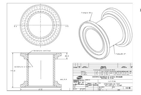
Fig. 4. Test structure made of stainless steel
