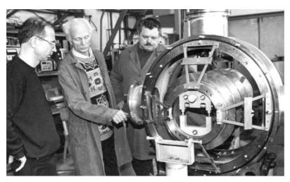
Veksler and Baldin Laboratory of High Energies. A new superconducting ion source with an electron-cyclotron resonance is produced for FLNR's IC-100 accelerator
