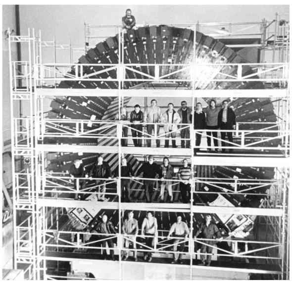
CERN, 30 October. Final ground installation of the barrel for the hadron calorimeter of the ATLAS set-up
