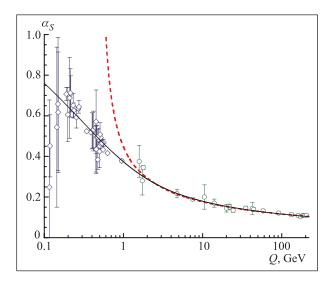
Summary of BS + APT extracted ( $\diamondsuit$ ) and high-energy ( $\circ$ ) data for  $\alpha_s(Q^2)$  against the three-loop analytic running coupling (solid curve), and its perturbative counterpart (dashed curve), both normalized at the  $Z_0$ -boson mass
