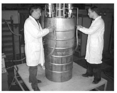
Laboratory of Particle Physics. Parts of the new accelerator for radiation technologies: pulse voltage formation system (left) and vacuum chamber with a high voltage line (right)
