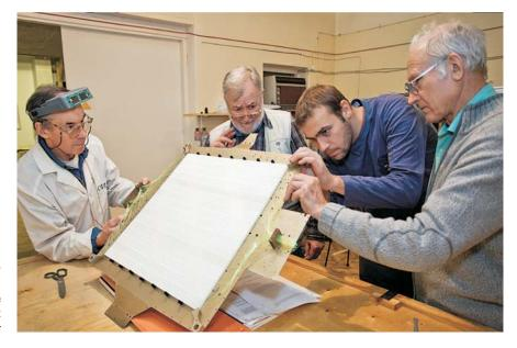
Dzhelepov Laboratory of Nuclear Problems. The assembly of the trigger module of the time-of-flight unit of the NUKLON detector
