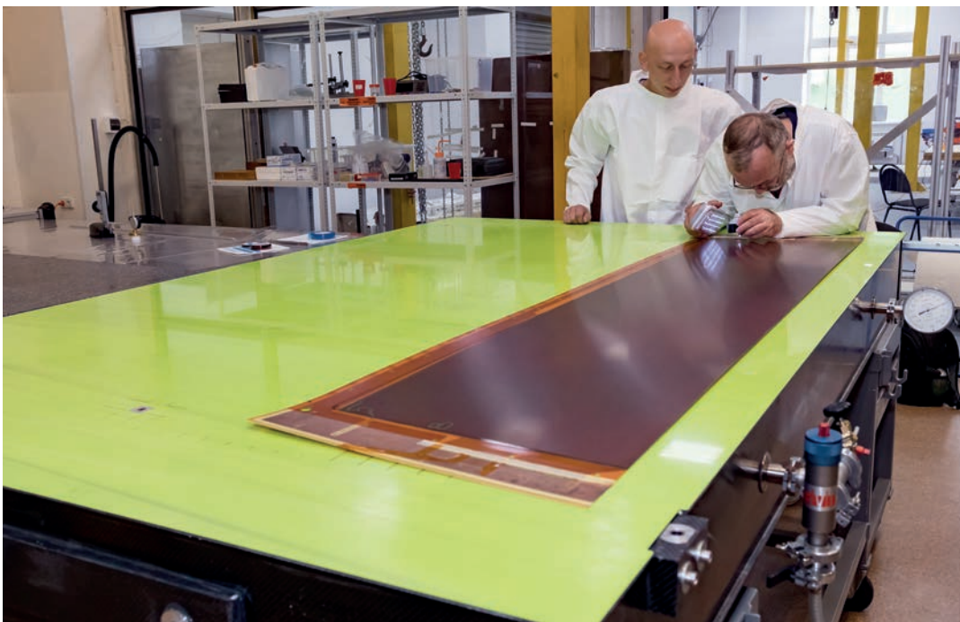
The Dzhelepov Laboratory of Nuclear Problems. Checking of the reading circuit plates of the Micromegas chambers for the ATLAS facility
