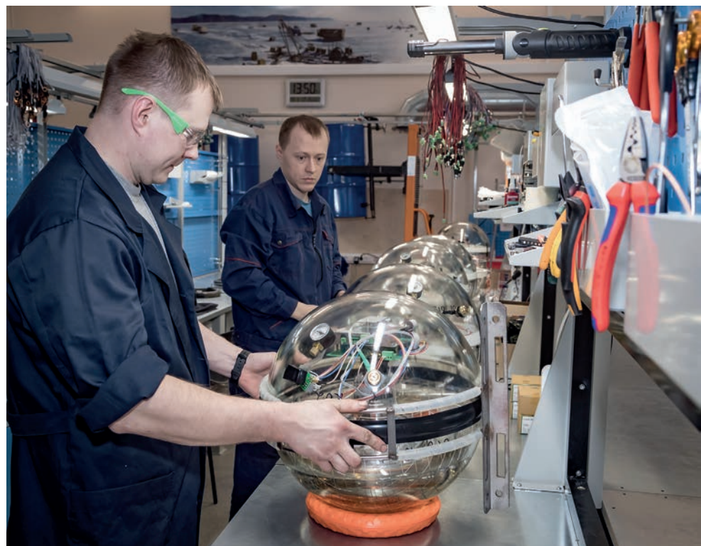
The Dzhelepov Laboratory of Nuclear Problems. Assembling optical modules for the Baikal-GVD project
