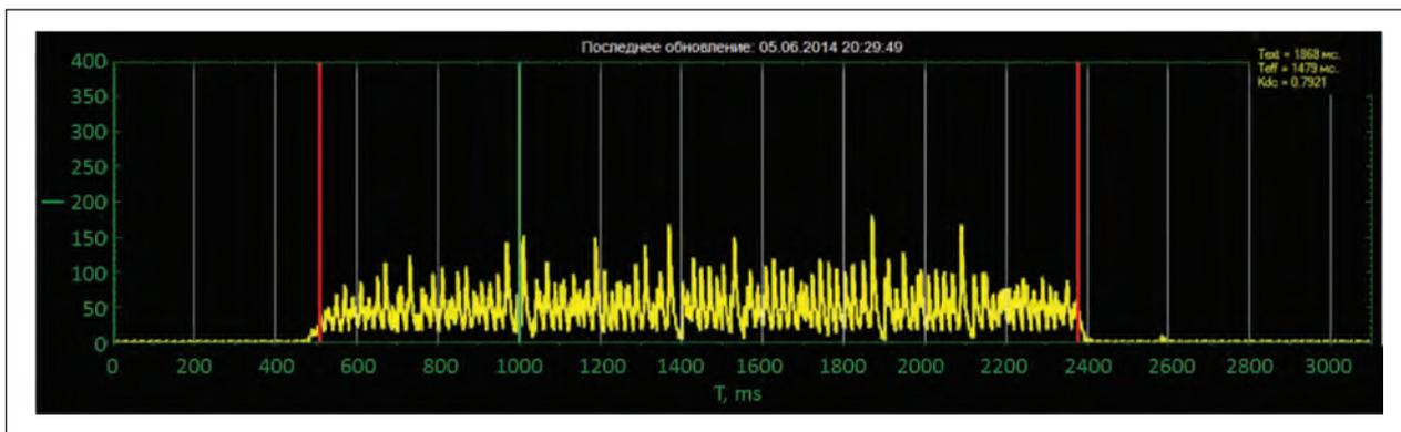
Fig. 2. Intensity time dependence of the extracted  $^{40}\text{Ar}^{16+}$  beam. Energy is 1.2 GeV/u, total ion number is  $1.5 \cdot 10^5$ , the spill duration is 2 s
