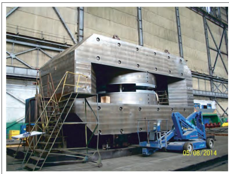
Fig. 1. The main magnet of the DC-280 cyclotron at the Novokramatorsk Machine-Building Plant
