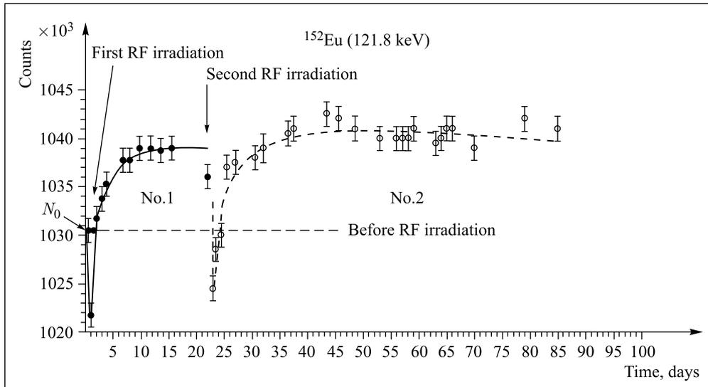
Fig. 7. Evolution of the 121.8 keV line intensity after two RF irradiations
