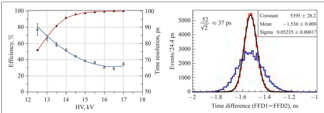
Fig. 3. Time resolution and efficiency of the MRPC strip for the time-of-flight system (left); time distribution between two identical prototypes of FFD (right)
