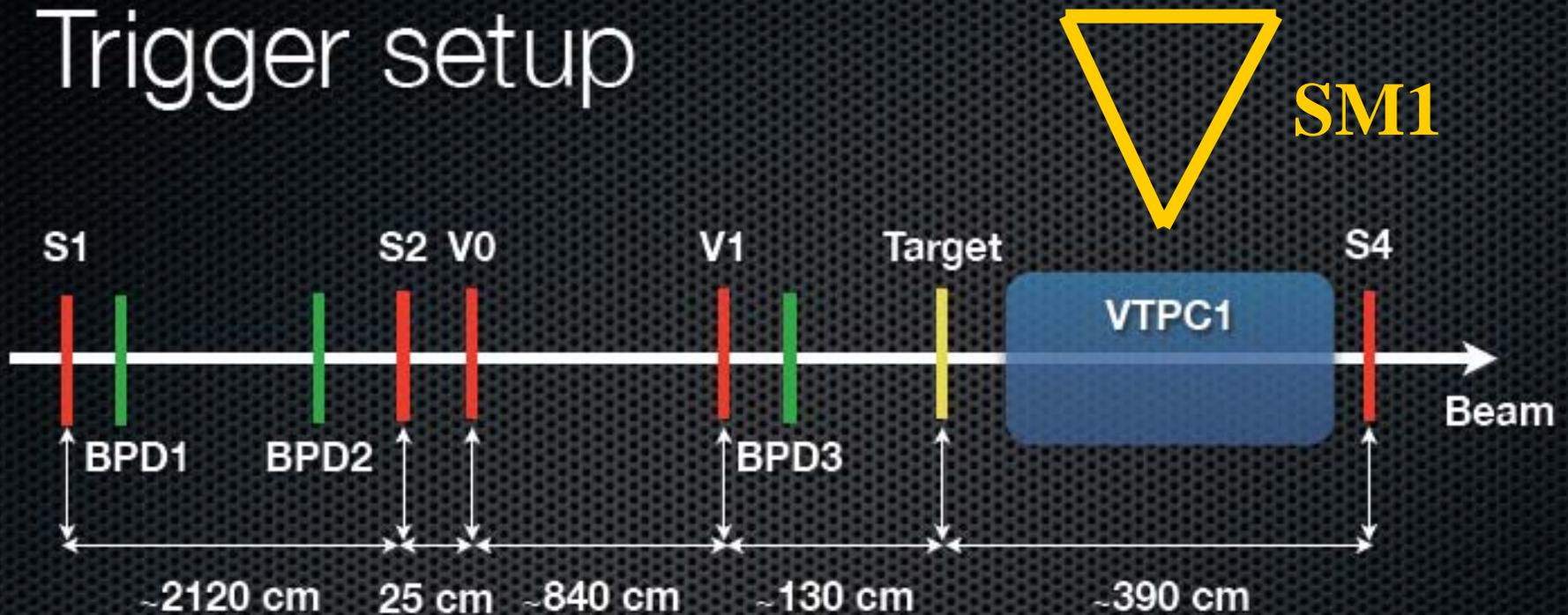
**Trigger definition: S1 & S2 &  $\overline{V0}$  &  $\overline{V1}$  &  $\overline{S4}$**
