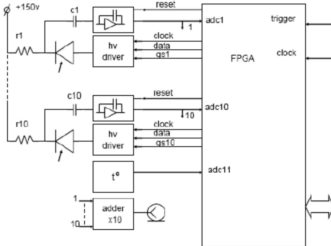
Fig.34 PSD front-end electronics, FEE.
