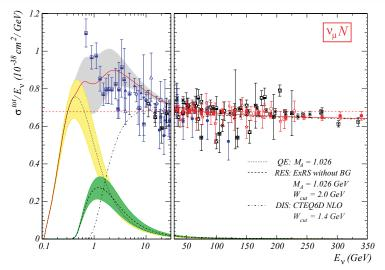
$\sigma^{tot}/E_{\nu}$ , for the muon neutrino charged-current total cross section as function of neutrino energy. The straight line is the average value  $(0.677 \pm 0.014) \times 10^{-38}$  cm<sup>2</sup>/GeV.
