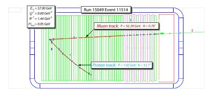
Typical examples of data events identified as  $\nu_{\mu} n \to \mu^{-} p$  (run 15049 event 11514). Long track is identified as negatively charged muon, short track is associated with proton.
