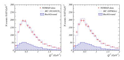
$\mathsf{Q}^2$  distribution in identified QEL events in MC and experimental data: comparison between DPMJet and NUANCE generators.
