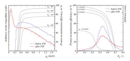
Distribution of leading proton momentum  $p_h$  and emission angle  $\theta_h$  before (dash-dotted line) and after (solid line) intra-nuclear cascade. Dashed lines show the reconstruction probability of proton track.
