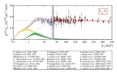
$\sigma^{tot}/E_{\nu}$ , for the muon antineutrino charged-current total cross section as function of neutrino energy. The straight line is the average value  $(0.334 \pm 0.008) \times 10^{-38}$  cm<sup>2</sup>/GeV.
