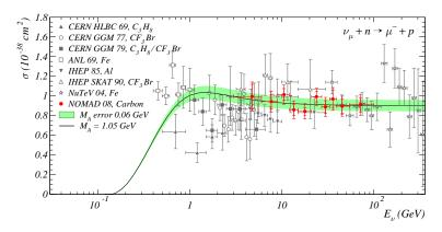
Comparison with previous experimental data extracted from the data on  $\nu_{\mu}$  scattering off heavy nuclei. The solid line and error band corresponds to the  $\textit{M}_{A}$  value obtained in the NOMAD experiment. Nuclear effects are included into calculations according to the standard relativistic Fermi gas model. The theoretical band corresponds to both statistical and systematical uncertainties.
