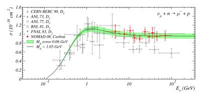
Comparison with previous experimental data from deuterium filled bubble chambers. The solid line and error band corresponds to the  $M_A$  value obtained in the NOMAD experiment. All experimental data are corrected to nuclear effects.
