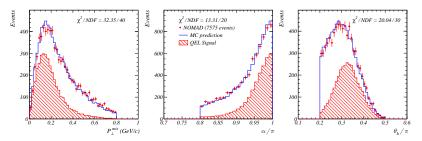
Missing transverse momentum  $P_{\perp}^{mis}$ , angle  $\alpha$  between the transverse components of the charged primary tracks and angle  $\theta_h$  between the proton momentum and z axis. Comparison of expected and experimental data distributions.
