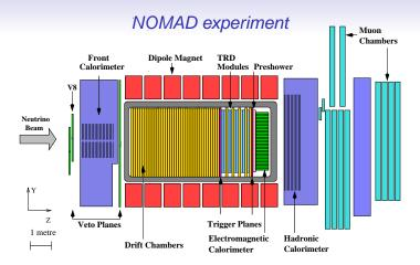
Drift Chambers (target and momentum measurement)
